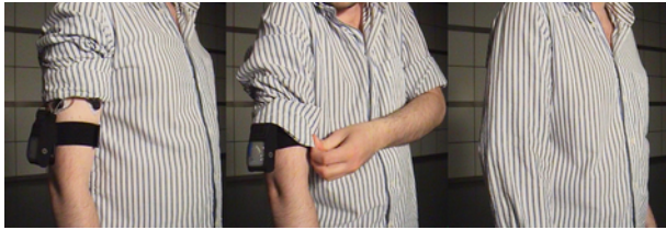
Figure 12: The Intimate Communication Armband worn on the upper arm.
