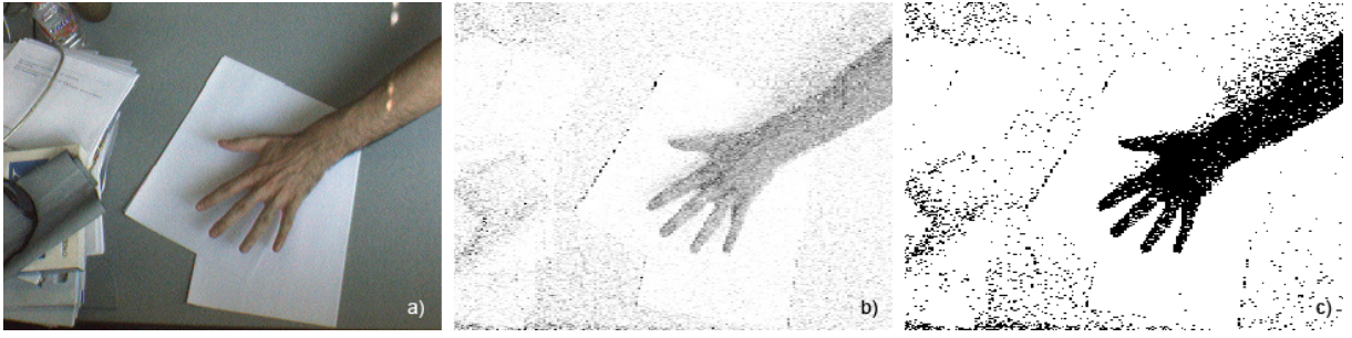
Figure 3: The CED metric: a) background model with hand, b) difference map with the CED metric not thresholded, c) thresholded.
