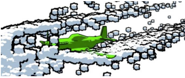
Figure 54: Clouds deflected by collisions with an airplane and interacting with the forces from the propellor.
