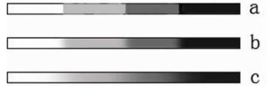
Figure 36: (a) Original 1D shading texture, (b) Bilinear filtering, (c) Blurred with the Gaussian function
