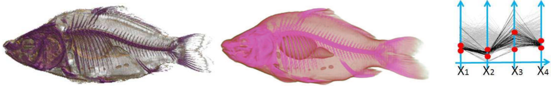
Figure 2.3: Rendering results generated by a gradient magnitude 2D TF (left) and by the presented parallel coordinates method (center). The TF design uses four parameters (right).
