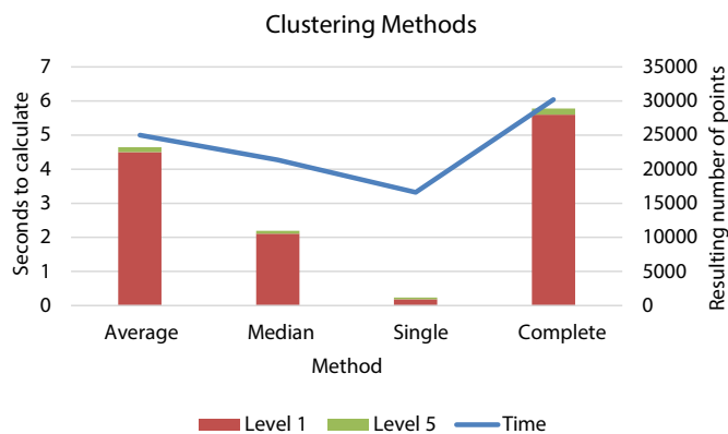
Figure 3.6: Number of atoms at levels 1 and 5 and building time, showing the number of resulting clusters for 2btv for level 1 (red) and 5 (green) as well as the time it takes to build the data structure using that method (blue).
