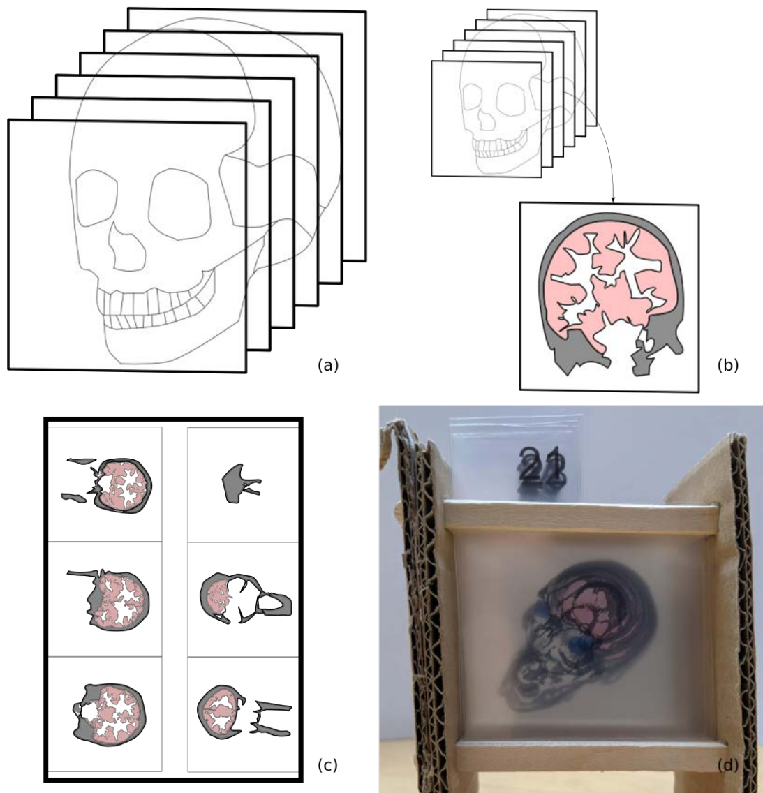
Figure 3.7: Concept of the Vologram workflow. (a) Users select a viewing direction and the image is resampled along the viewing axis. (b) In a regular interval, images are sampled along the viewing direction and mapped to a rectangular plane. (c) Sub-images are arranged on a printable page. (d) The stencil is printed out and cut along the predefined lines. Images are assembled in order, in a constant distance. This creates a 3D hologram-like appearance.
