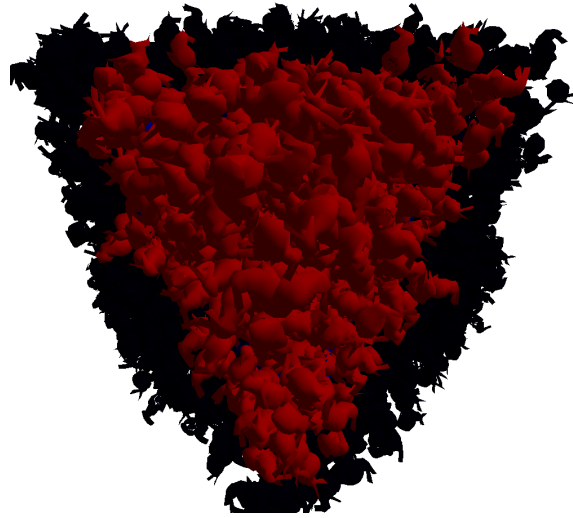
Figure 4.3: Front view of the camera. The red bunnies are the occluders, the blue bunnies occludees. The brighter the blue, the lower is the level of visibility and therefore their polygon count.
