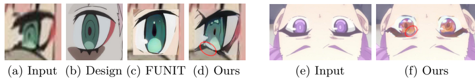
Figure 5.17: Redrawing Limitations. Our method vastly improves upon existing work on handling occlusions; however, it still can struggle with uncommon scenarios (top). As it was trained mostly with upright eyes, fails if input is not pre-rotated to upright position (bottom).
