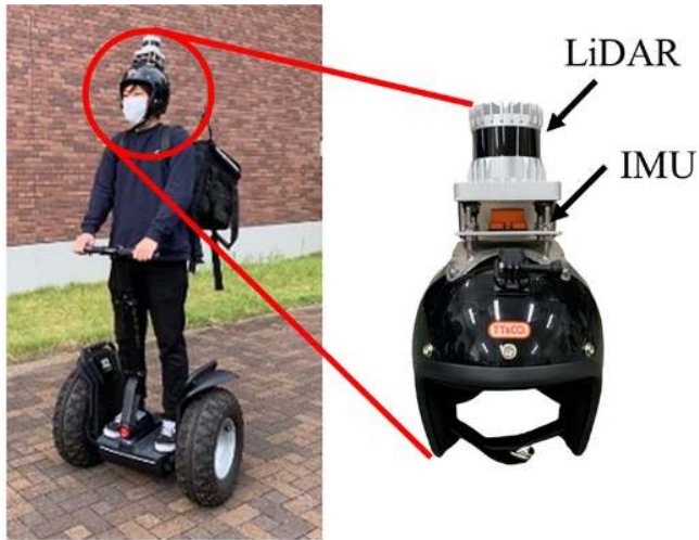
Overview of experimental smart helmet
